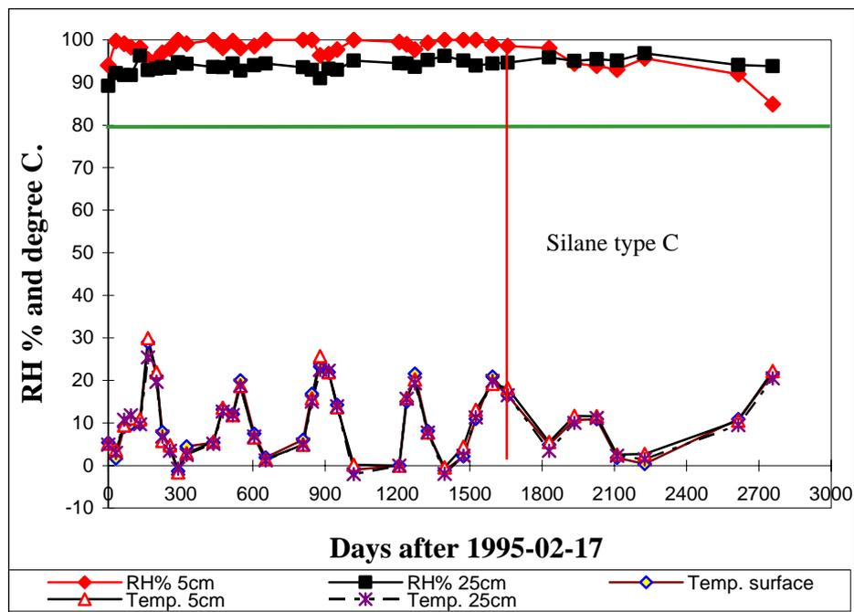
Fig. 6. Relative humidity and temperature during 7 years measurements. Silane type C was applied the column after about 1600 days. Note that 5 cm from the surface the relative humidity reduces after the impregnation with silane.
