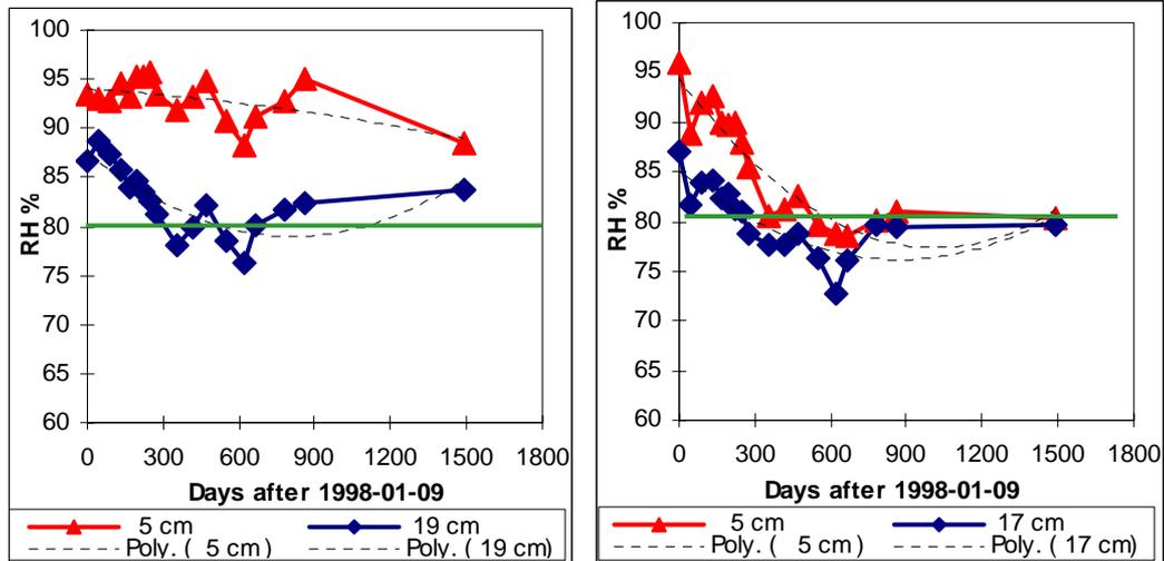
Fig. 11. Relative humidity 5 cm and 19 cm from outer surface in a reference (left figure) and a location treated with silane type A (right figure) after 1493 days, DNV
