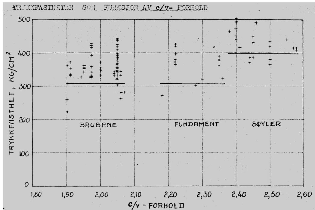
Figure 5: compressive strength from control specimens during the construction period. X-axis is cement/water –relation and Y-axis is compressive strength (kg/cm<sup>2</sup>).
