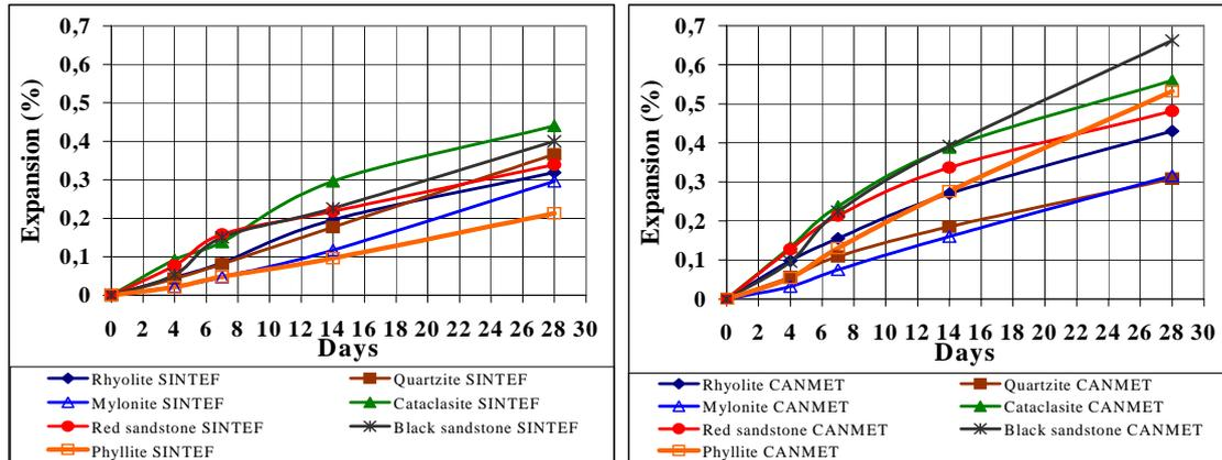
Fig. 2: Expansions of AMBT, SINTEF (left figure) and CANMET (right figure)
