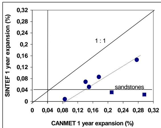
Fig. 5: Correlation of concrete prism expansions between SINTEF and CANMET
